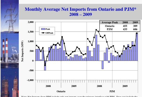
Note: Net Imports from PJM include only net imports over the primary interface with PJM. Does not include the Neptune line or Linden VFT shown later. -142-
