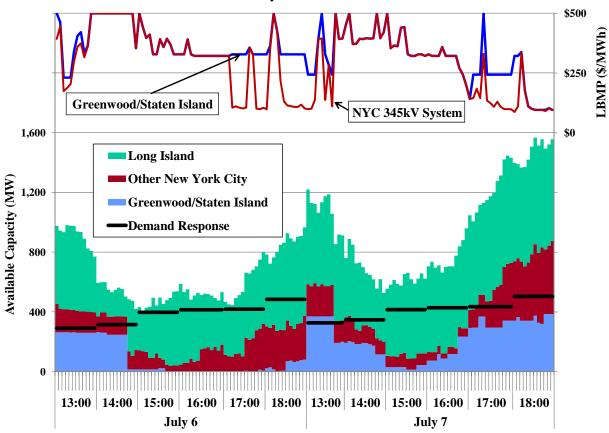
**Figure 51: Real-Time Prices and Available Capacity in Demand Response Activations** July 6 & 7, 2010
