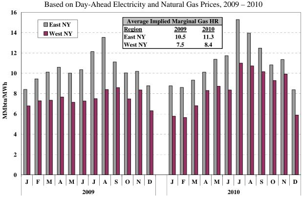
**Figure 2: Average Implied Marginal Heat Rate** Based on Day-Ahead Electricity and Natural Gas Prices, 2009 – 2010
