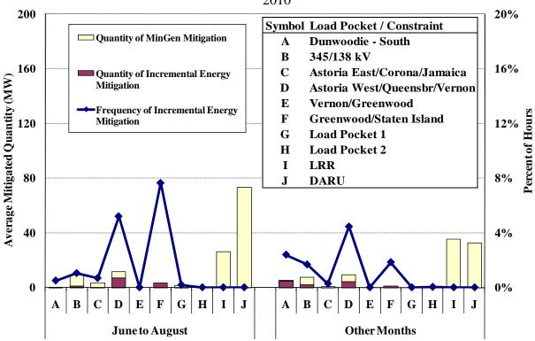
**Figure 20: Frequency of Day-Ahead Mitigation in the NYC Load Pockets** 2010
