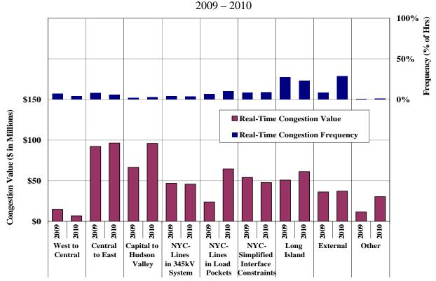
Figure 40: Real-Time Congestion by Transmission Path
