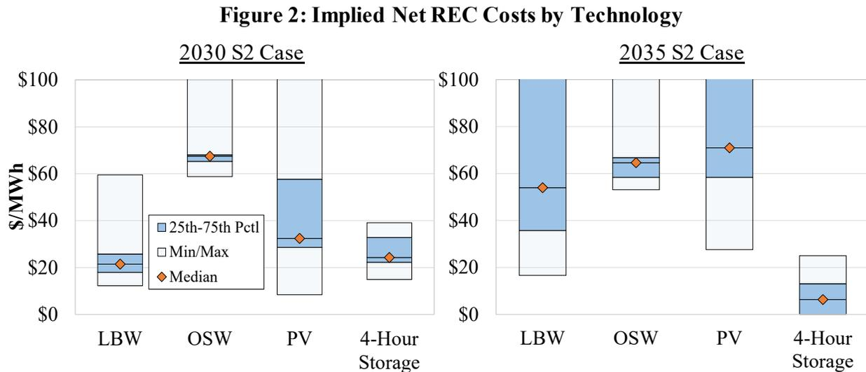
Figure 2 shows that the net REC costs vary significantly by technology and generally rise from 2030 to 2035 as large amounts of each resource enter and a higher share of each is sited at over-saturated locations. The one notable exception is the 4-hour storage resource.
