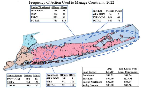
Figure A-61: Constraints on the Low Voltage Network on Long Island
