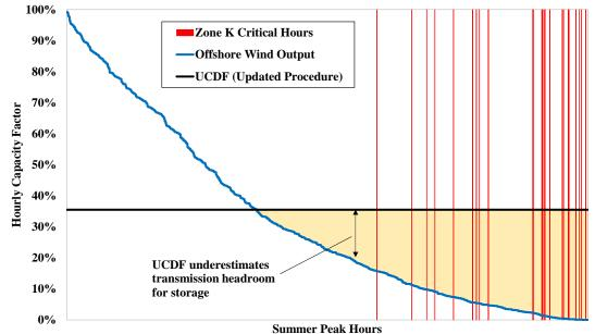
Figure 16: Long Island Offshore Wind Hourly Output and UCDF in Critical Hours
