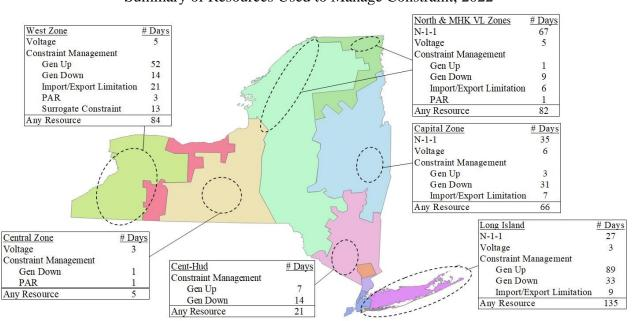
Figure A-60: Constraints on the Low Voltage Network in New York Summary of Resources Used to Manage Constraint, 2022
